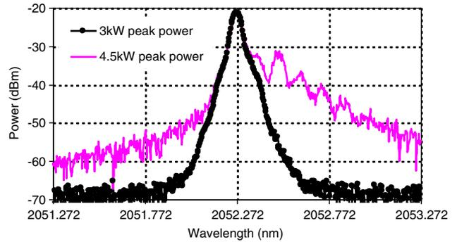
Fig. 6. (Color online) Zoom-in spectra of the amplified laser pulses at  $\sim 3$  kW peak power (black) and  $\sim 4.5$  kW peak power (pink). Stimulated Brillouin scattering appeared when the peak power was 4.5 kW.
