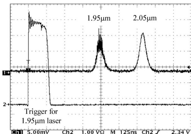
Fig. 2. Typical temporal profiles of a pump and gain-switched pulse for trace #1, and pump trigger for trace #2.
