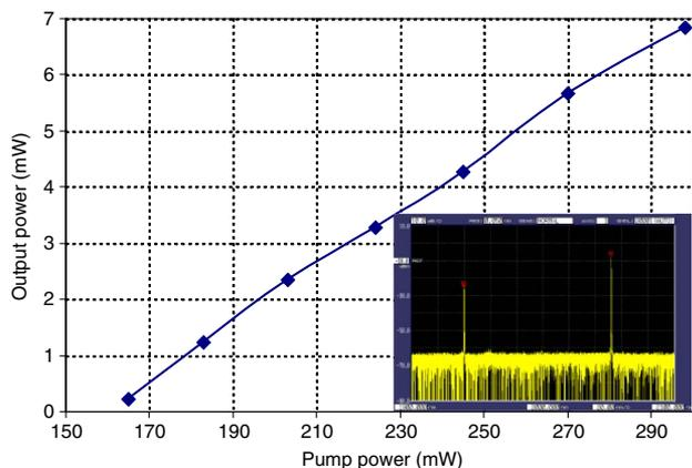
Fig. 1. (Color online) Laser output power versus launched pump power. Inset: spectrum of the pump pulses and signal pulses.
