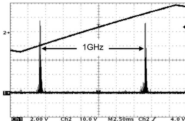
Fig. 3. Scanning FP interferometric spectrum of the gain-switched Ho-doped fiber laser verifying single-frequency operation.
