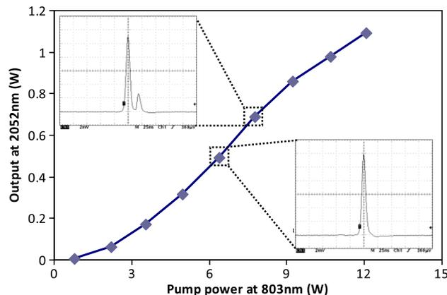
Fig. 4. (Color online) Output power extracted from the fiber amplifier. Insets: temporal profiles of the amplified pulses at average powers of 500 and 750 mW, corresponding peak power of 3 and 4.5 kW.
