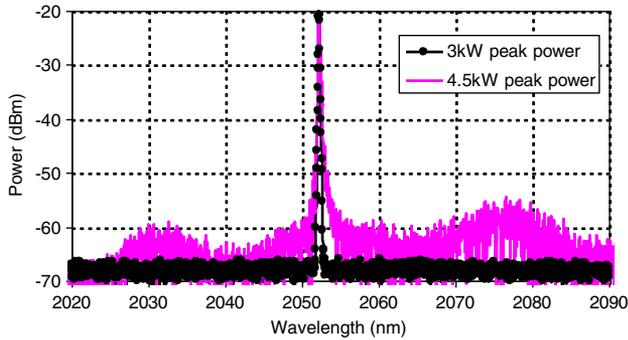
Fig. 5. (Color online) Optical spectra of the amplified laser pulses at  $\sim 3$  kW peak power (black) and  $\sim 4.5$  kW peak power (pink). MI sidebands appeared when the peak power was 4.5 kW.
