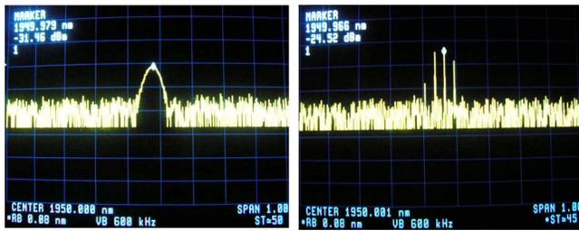
Fig. 2. (Color online) Laser spectra of the DBR fiber laser in cw (left) and  $Q$ -switched (right) modes. The four peaks in the graph on the right correspond to four sequential  $Q$ -switched pulses when the Hewlett Packard OSA was scanning across the laser wavelength.
