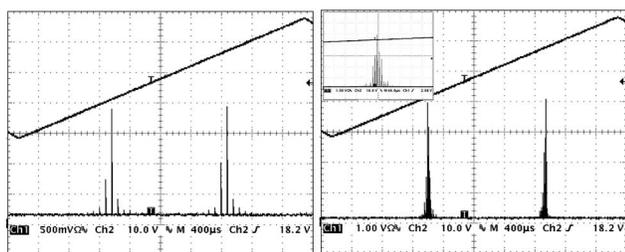
Fig. 5. Laser spectrum over one free spectral range (FSR  $\sim 800$  MHz) of an FP interferometer that verified single-frequency operation of the all-fiber  $Q$ -switched laser at 12.5 (left) and 125 (right) kHz. The inset in the right graph shows a zoom-in spectrum.
