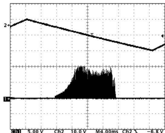
Fig. 6. Temporal profile of the laser intensity when the laser wavelength was swept over 200 nm in 16 ms.
