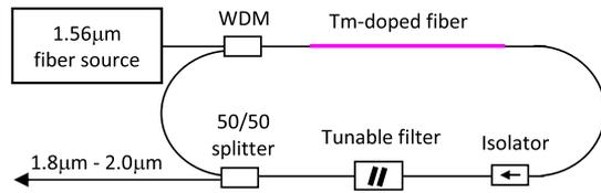
Fig. 3. (Color online) Schematic diagram of an all-fiber wavelength-swept laser near  $2 \mu\text{m}$ .
