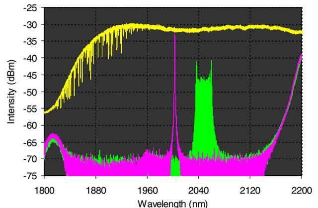
Fig. 2. (Color online) The FFP-TF is characterized by a mid-IR supercontinuum fiber source; yellow (upper) trace, supercontinuum spectrum; pink (lower) trace, transmission spectrum with a constant voltage; and green (middle) trace, transmission spectrum with a sawtooth voltage.
