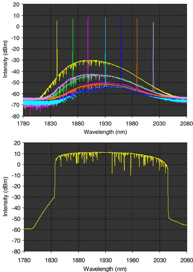
Fig. 4. (Color online) Typical laser spectra when constant voltages (upper) and a swept voltage (lower) were applied to the tunable filter. In the lower graph, some wavelengths were not caught by the OSA during the scans due to no synchronization.
