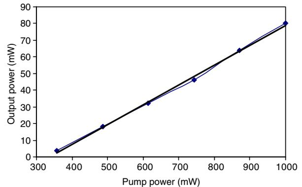
Fig. 5. (Color online) Output power of the laser at 1930 nm as a function of the pump power.
