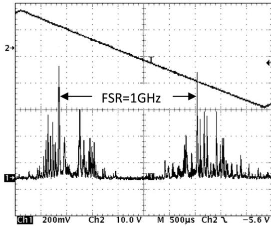
Fig. 7. Laser spectral linewidth is measured by using a high-resolution scanning FP interferometer with an FSR = 1 GHz and a finesse of  $\sim 270$ .
