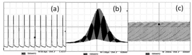
Fig. 3. Tm–Ho-fiber laser pulse trains. (a) *Q*-switching. (b) *Q*-switched mode-locking. (c) Mode-locking.
