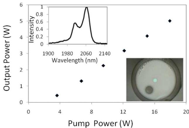
Fig. 1. Tm–Ho-codoped cw fiber laser output power as a function of 798-nm pump power. Top-left inset is a typical ASE spectrum of Tm–Ho-codoped silicate fiber with cladding pump at  $\sim 800$  nm. Bottom-right inset is the microscope image of the fiber facet.
