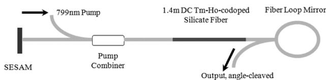
Fig. 2. Schematic of mode-locked Tm–Ho-codoped silicate fiber laser.
