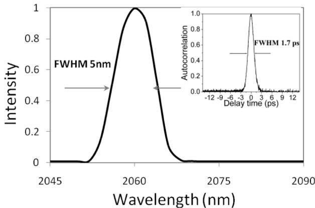
Fig. 4. Mode-locked Tm–Ho-fiber laser spectrum. Inset is the autocorrelation trace of the mode-locked laser pulses.
