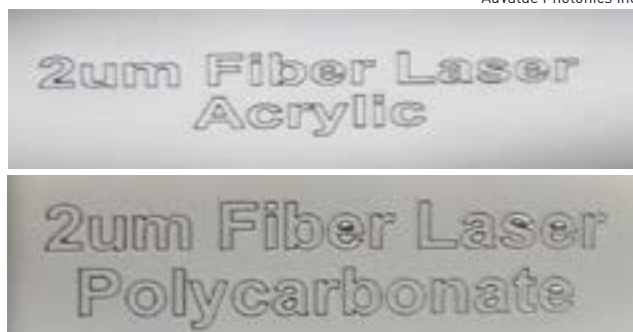
Laser marking on transparent plastic materials with a Q-switched 2 \mu\text{m} fiber laser.
