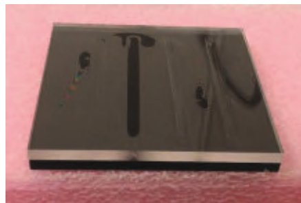
FIGURE 2. Clear (top) and black (bottom) PMMA plates bonded together through the laser-produced welding track (the dark line slightly on the left of the sample). In this case, the CW 2μm laser beam actually entered the sample from the black piece, not from the clear piece.
