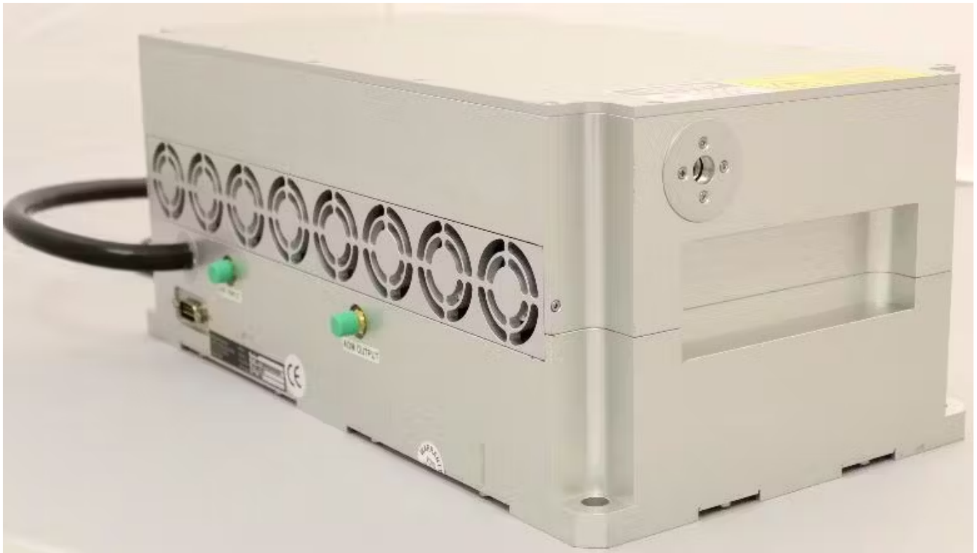
FIGURE 4. The all-fiber monolithic pulsed laser system delivers >1 mJ pulses from a compact package comprised of commercially available fiber-optic components and specialty doped gain fibers.
